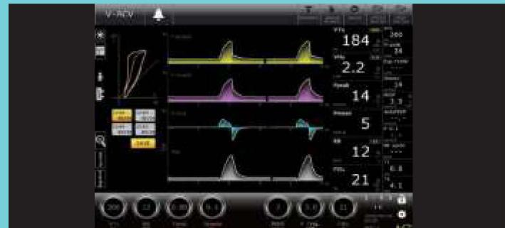
Patient's circuit and intubation, ET tube, leakage, etc. may cause patient to have pressure in the lung and measurement error of the equipment. This function allows the ventilator to be controlled by measuring the direct pressure by insert a catheter into the intubation tube. The airway pressure displayed on the ventilator is higher than the set value.
